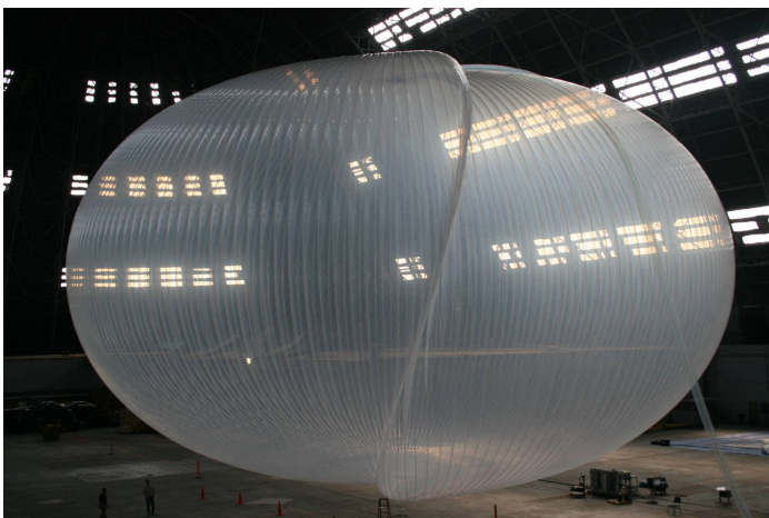
Scaled model (30 m diameter) of NASA superpressure balloon (Courtesy of NASA BPO)
